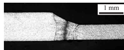
(a) 270 MPa (1.2 mm t ) / 270 MPa (0.65 mm t ), Welding speed: 8.5 m/min
